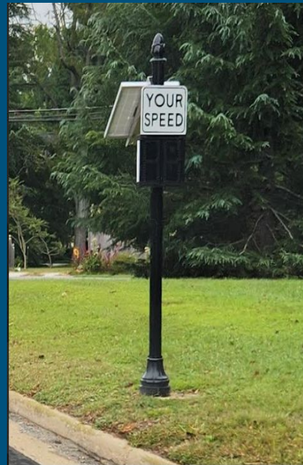
*Above- Pole-mounted speed display in Warsaw VA
